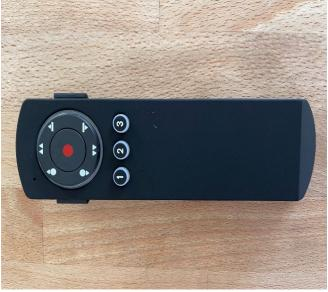
The Brick is the Control box which is connected to the motor using the cable via the larger 8 PIN connector on the Brick and Motor. The Wireless controller has a Red button for setting the controller to enable memory settings and control one motor or sync two motors together (see below). The left round icons control the head/back motions (up and down) and the right flat icons control the foot section (up and down). There are three memory buttons to memorize the adjustable settings.
